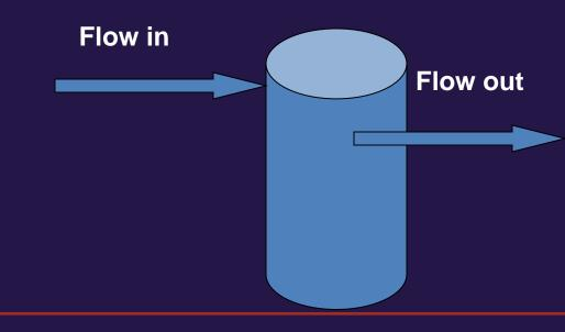
Question: A water reservoir that is 20 ft diameter with a depth of 16 ft needs to be filled up. If the well is pumping at 200 gpm, how long will it take to fill in minutes? In hours?
