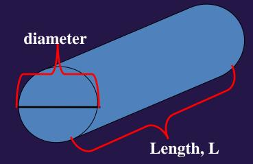
Tank Volume = Area x Height Area =  $\pi$  x r<sup>2</sup> =  $\pi/4$  x D<sup>2</sup> Volume =  $\pi$  x r<sup>2</sup> x H =  $\pi/4$  x D<sup>2</sup> x H
