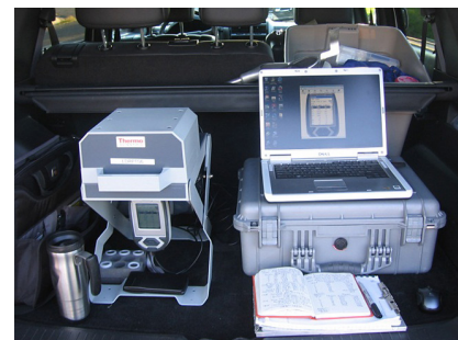
On-site analysis of metals with XRF
