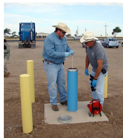
Nested wells for two transmissive zones
