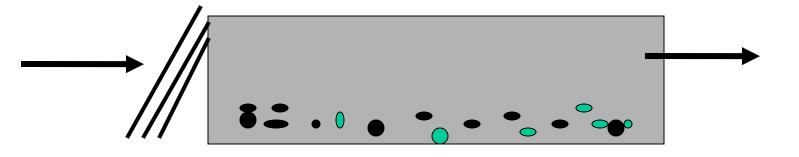
HEAVY, INORGANIC MATERIAL REMOVED IN GRIT CHAMBER (BY REDUCING THE VELOCITY)
