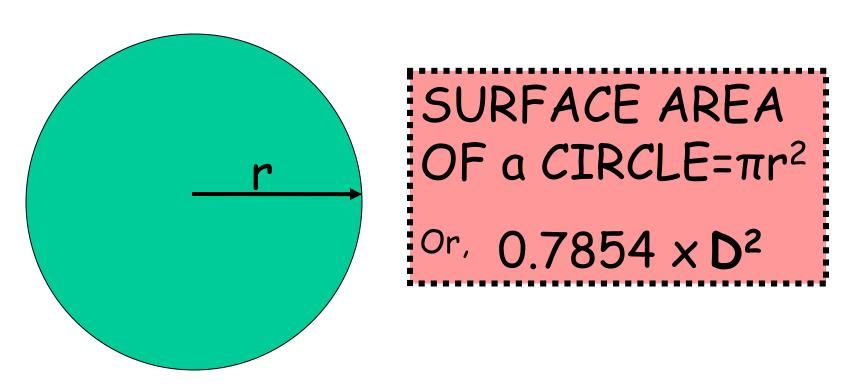
Example: What is the surface area of a circular tank that is 65' in diameter:  $5A = 0.7854 \times 4225 \text{ sq-ft} = 3317 \text{ sq-ft}$
