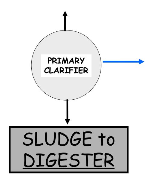
SETTLED EFFLUENT TO SECONDARY TREATMENT
