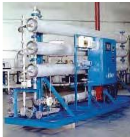
Figure 15.17 - Reverse Osmosis Unit (courtesy SpinTek Corp.)
