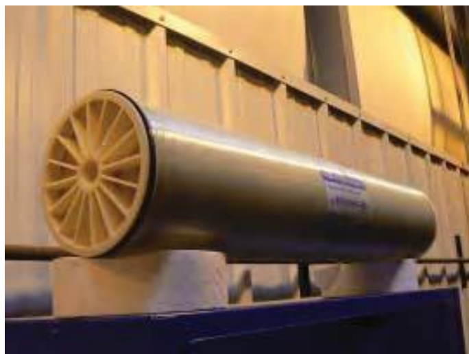
Figure 15.13 - FilmTec Spiral Wound RO element (S. Hanson photo file)
