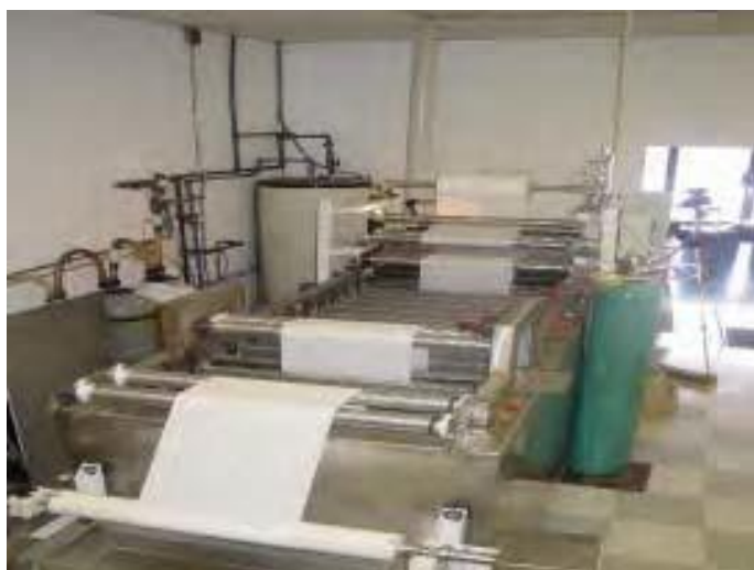
Figure 15.10 Spiral Wound element rolling device (Separation Systems Technology – S. Hanson photo file)
