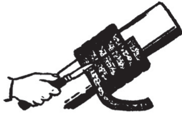
CUT AND FLATTEN PACKING
