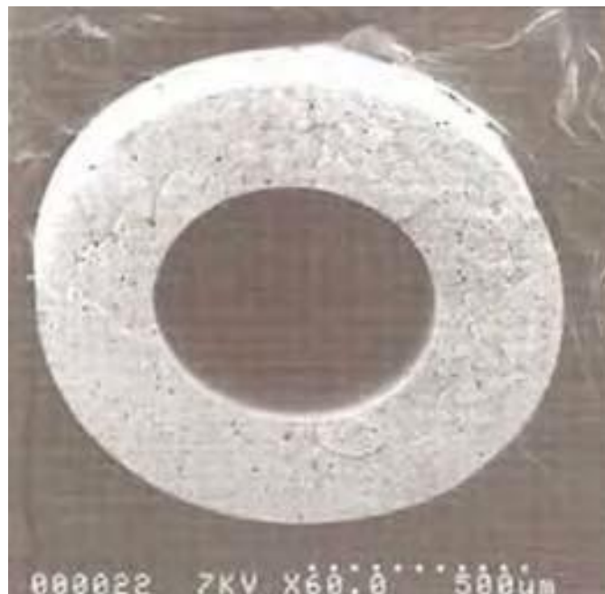
Figure 15.9 - Cross Section of Hollow-fiber Microfilter (Courtesy of Pall Corp.)
