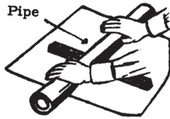
CUT AND FLATTEN PACKING
