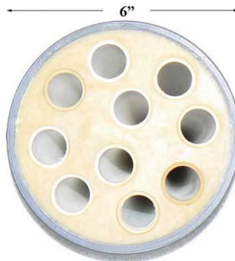
Figure 15.8 - End view of MF tube bundle (Siemens Water Technology Memtek membrane, S. Hanson photo file)
