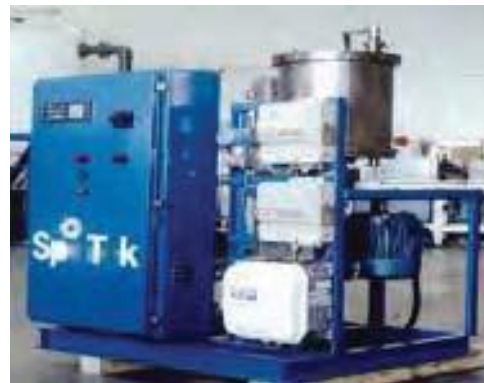
Figure 15.15 - Centrifugal Ultrafiltration Unit (courtesy SpinTek Corp.)
