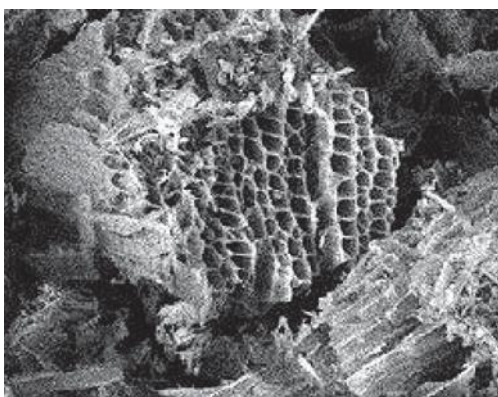
Figure 15.1 - Activated carbon, as viewed by an electron microscope
