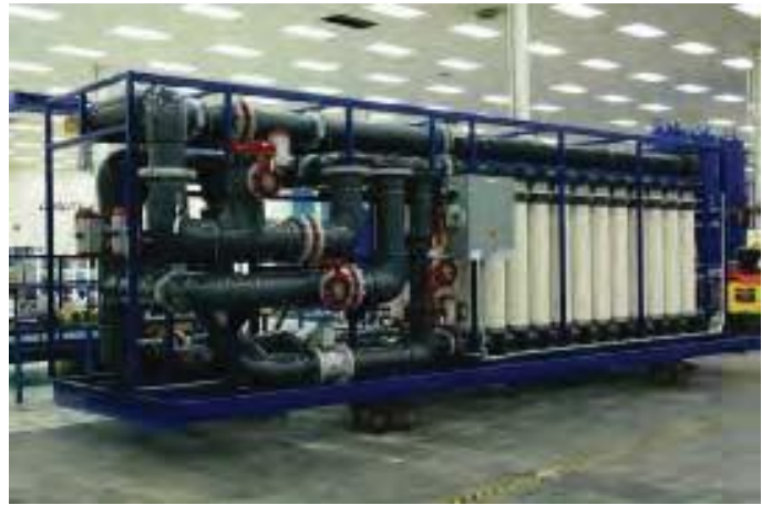
Figure 15.14 –440 GPM MF System (courtesy of Siemens Water)
